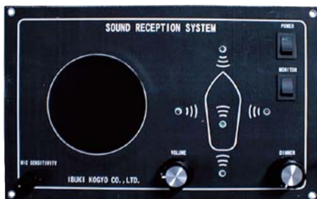
SRS Control Panel
