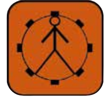
ENGINEER'S ALARM ENGINE ROOM
